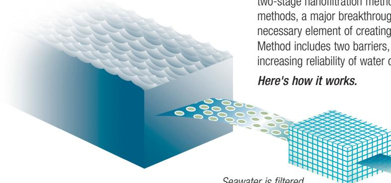
*Seawater is filtered to remove suspended materials and is then pumped to Stage 1.*
