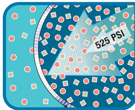
**Stage 2:** Water from Stage 1 – seawater with only smallest 12% of salt molecules – is pumped under lower pressure through second nanofiltration membrane, which blocks passage of almost all remaining salts.
