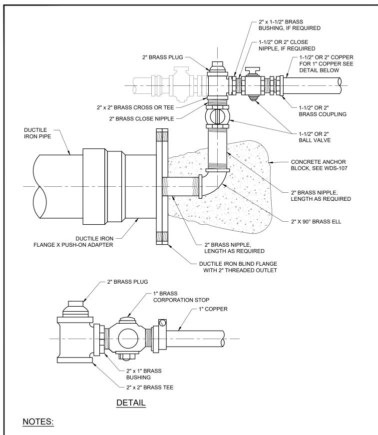
1. ALL BRASS NIPPLES AND FITTINGS SHALL BE GREASED AND WRAPPED. NO CONTACT WITH CONCRETE WILL BE ALLOWED.
